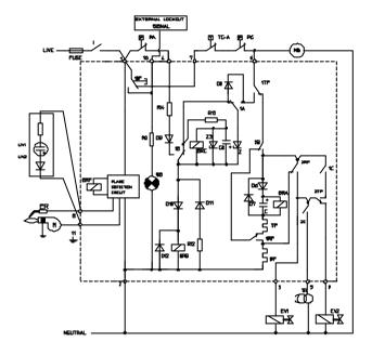
BF. Lockout and postpurge thermal Burner casing BRA. Granted prepurge relay MB: Burner motor BRB: PA: Air pressure switch Operation relay BRC: Safety time relay PG. Gas pressure switch BRF: Flame detection relay SB: Lockout signal Detection probe Thermal programmer TC-A: First gas valve Thermostats EV2: Second gas valve UV1 UV2: Phototube
